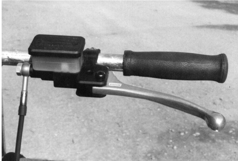
Abb.9 Hydraulikhebel figure 9 hydraulik brake lever
