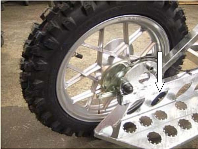
Abb.5 Trommelbremse figure 5 drum brake
